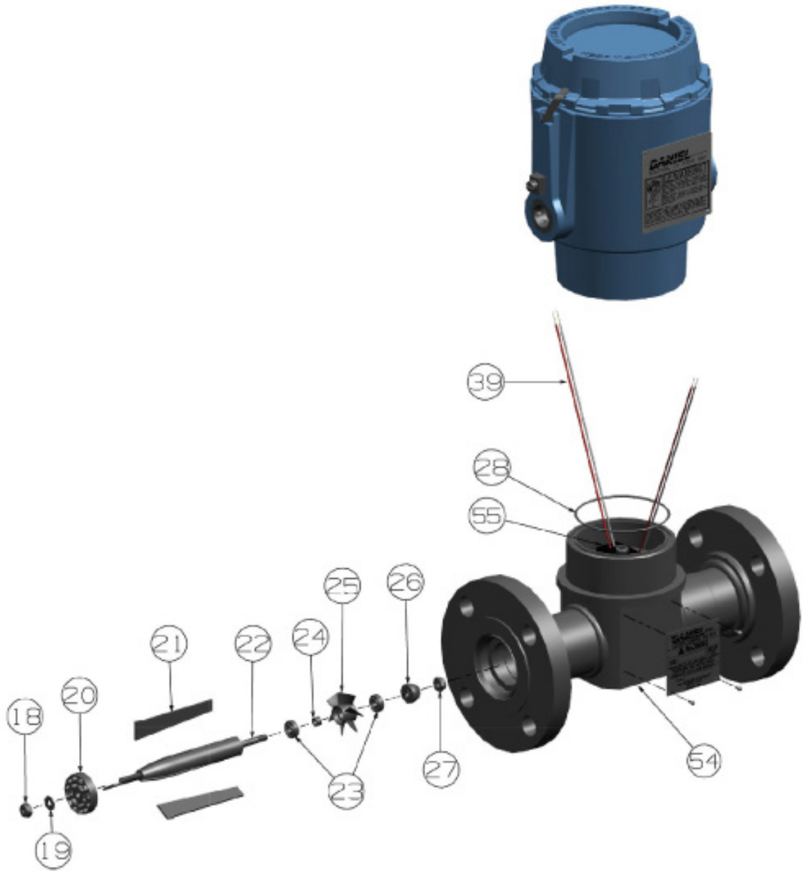
FIGURE 1-4: PART IDENTIFICATION FOR AN NPS 1.5 THROUGH 2 LTM
