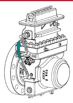
7. Rotate the Upper Plate Carrier Shaft (7) located in the Top (14) until the Plate Carrier (8DM or 8DMC) stops against the Sealing Bar (9, 9HP).
