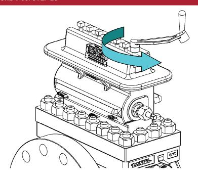
29. Once the Clamping Bar Screws (11) are loose, it may be necessary to use the Operating Wrench (2) to tap against the Sealing Bar (9 or 9HP) freeing it from the Top (14).
