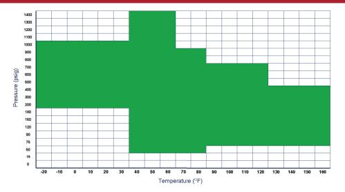
Pressure (psig) v. Temperature (°F) CARBON DIOXIDE GREASE - TYPE 3 - Part Number:1-213-04- 101 OPTIMUM SEALING RANGE WITH NITROGEN FOR A 3" ANSI 600 SENIOR FITTING UNDER LABORATORY CONDITIONS. Colored coordinate boxes indicate no detectable leakage at that Temperature and Pressure for 30 minutes.
