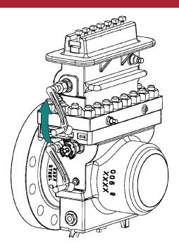
7. Rotate the Upper Plate Carrier Shaft (7) located in the Top (14) until the Plate Carrier (8DM or 8DMC) stops against the Sealing Bar (9 or 9HP).
