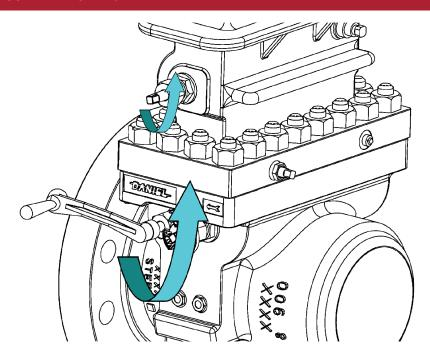
6. Move the Operating Wrench (2) from the Lower Plate Carrier Shaft (6) located in the Body (4) on the Upper Plate Carrier Shaft (7) located in the Top (14).
