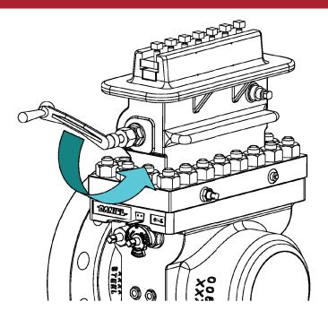
8. Close the Equalizer Valve (1) with the Operating Wrench (2).
