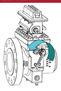
10. Open the Bleeder Valve (10B) with the Operating Wrench (2).
