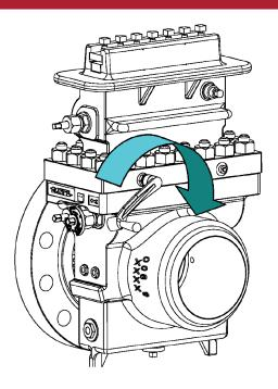
9. Using the Operating Wrench (2) rotate the Slide Valve Shaft (5) until it stops and the CLOSED position specified on the Indicator Plate (5A) is in line with the Indicator Pointer (5B).
