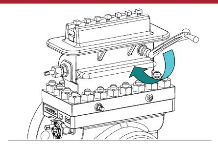
39. Open the Equalizer Valve (1) one-half to two turns with the Operating Wrench (2).
