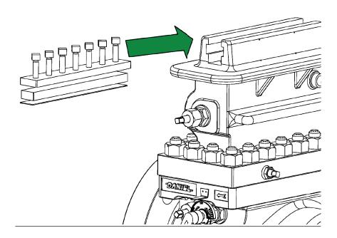
22. Tighten each Clamping Bar Screw (11) located on the Clamping Bar (12 or 12HP) (Reference: Torque information.)
