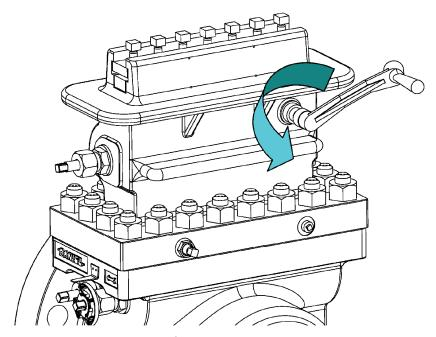
Step 47 and 48 are ONLY required for Seniors equipped with grease assisted, metalto- metal slide valves. Personnel operating the Daniel Senior Orifice Fitting equipped with O-Ring seal "soft seat" design slide valves skip to step 49.
