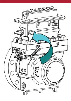
2. Wait several seconds while the pressure in the Top (14) equalizes to that of the Body (4).
