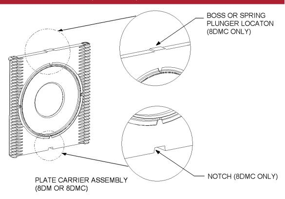
The diagram below depicts the proper orientation of the Plate Carrier (8DM or 8DMC) assembly prior to lowering it into the measurement position in the Senior.
