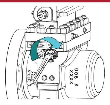
30. Rotate the Upper Plate Carrier Shaft (7) with the Operating Wrench (2) in the direction to lower the Orifice Plate Carrier (8DM or 8DMC) into the Body (4).
