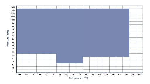
Pressure (psig) v. Temperature (°F) SOUR GAS GREASE - TYPE 2 - Part Number:1-213-04-102 OPTIMUM SEALING RANGE WITH NITROGEN FOR A 3" ANSI 600 SENIOR FITTING UNDER LABORATORY CONDITIONS. Colored coordinate boxes indicate no detectable leakage at that Temperature and Pressure for 30 minutes.
