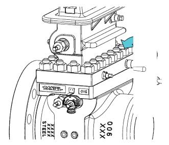
26. Return the stem to the Grease Gun (23) and begin turning it clockwise by hand into the Grease Gun (23) until resistance is felt. Once this is done, use the supplied Operating Wrench (2) to continue to turn the stem at a rate of 4 to 6 turns per minute.
