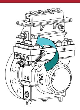
40. Wait several seconds for the Top (14) to reach pressure equilibrium with the line pressure contained in the Body (4).
