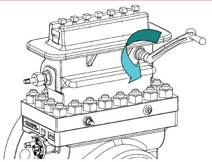
Steps 35 and 36 are ONLY required for Seniors equipped with grease assisted, metal-to-metal slide valves. Personnel operating the Daniel Senior Orifice Fittings equipped with O-Ring seal "soft seat" design slide valves skip to step 37.
