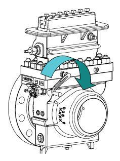
Using the Operating Wrench (2) rotate the Slide Valve Shaft (5) until it stops and the CLOSED position specified on the Indicator Plate (5A) is in line with the Indicator Pointer (5B).
