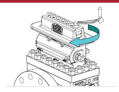
38. Tighten each Clamping Bar Screw (11), located on the Clamping Bar (12 or 12HP) (Reference: Torque information.)
