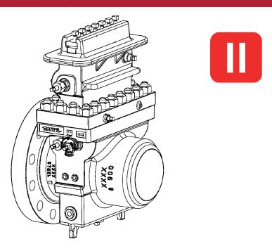
41. Using the Operating Wrench (2), rotate the Slide Valve Shaft (5) to the OPEN position.
