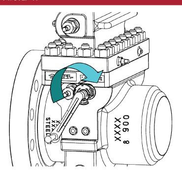
42. Rotate the Upper Plate Carrier Shaft (7) located in the Top (14) with the Operating Wrench (2) in the direction to lower the Orifice Plate Carrier (8DM or 8DMC) into the Body (4).
