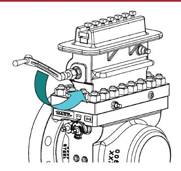
16. Slide the Clamping Bar (12 or 12HP) containing the Clamping Bar Screws (11), the Sealing Bar (9 or 9HP) from the Top (14).
