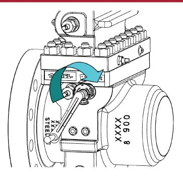
4. Rotate the Lower Plate Carrier Shaft (6), located on the Body (4), using the Operating Wrench (2) in a direction that will move the Plate Carrier (8DM or 8DMC) out of the Body (4) into the Top (14).
