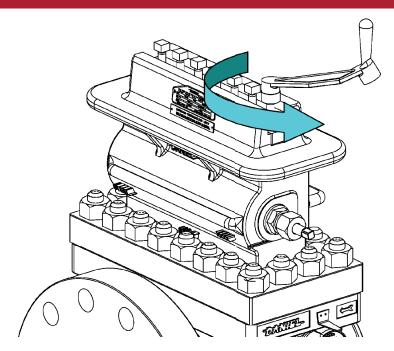
15. Once the Clamping Bar Screws (11) are loose, rotate the Upper Plate Carrier Shaft (7) located in the Top (14) with the Operating Wrench (2), until the Plate Carrier (8DM or 8DMC) taps against the Sealing Bar (9 or 9HP) freeing it from the Top (14).
