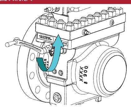
5. Continue to rotate the Lower Plate Carrier Shaft (6) located on the Body (4) until the Upper Plate Carrier Shaft (7) located in the Top (14) begins to rotate.
