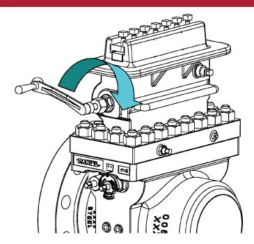
43. Rotate the Lower Plate Carrier Shaft (6) with the Operating Wrench (2) until the Orifice Plate Carrier (8DM or 8DMC) cannot be lowered further.
