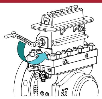
30. Slide the Clamping Bar (12 or 12HP) containing the Clamping Bar Screws (11), the Sealing Bar (9) from the Top (14).
