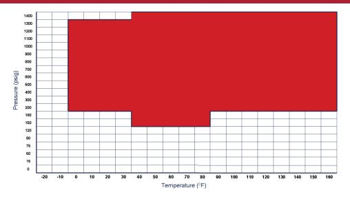
Pressure (psig) v. Temperature (°F) STANDARD GREASE - TYPE 1 - Part Number: 1-213-04-001 OPTIMUM SEALING RANGE WITH NITROGEN FOR A 3" ANSI 600 SENIOR FITTING UNDER LABORATORY CONDITIONS. Colored coordinate boxes indicate no detectable leakage at that Temperature and Pressure for 30 minutes.
