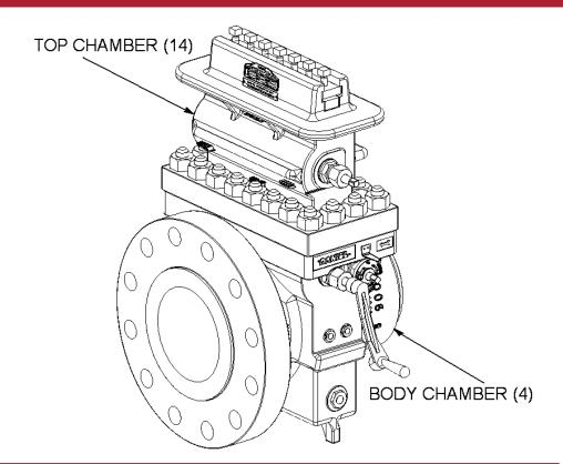
Therefore, using a Senior may eliminate the need for bypass piping, valves, and other fittings necessary with conventional orifice fitting installations. Maintenance technicians can replace and repair all parts of the Senior. including the slide valve assembly, without removing the Body (4) from the line (refer to Maintain).
