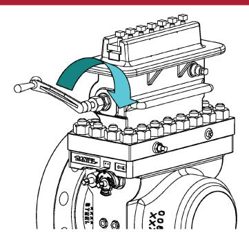
31. Rotate the Lower Plate Carrier Shaft (6) with the Operating Wrench (2) until the Orifice Plate Carrier (8DM or 8DMC) cannot be lowered further.
