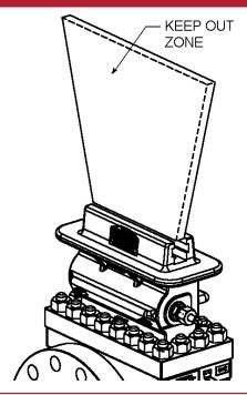
(7) Daniel Senior Orifice Fitting shown in vertical position. The KEEP OUT ZONE includes the plate carrier slot opening of the Top (14) even when the Senior is positioned horizontally (laying on its side).
