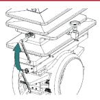
7. Rotate the Upper Plate Carrier Shaft (7) located in the Top (14) until the Plate Carrier (8DM) stops against the Sealing Bar (9).
