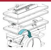
9. Using the Operating Wrench (2) rotate the Slide Valve Shaft (5) until it stops and the CLOSED position specified on the Indicator Plate (5A) is in line with the Indicator Pointer (5B).
