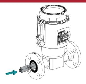
6. Install the sleeve and retainer ring in the groove in the upstream end of the housing bore. Tang side of the retainer ring is to be inserted last to provide for future disassembly.
