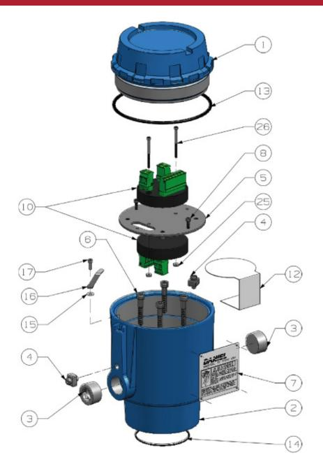
TABLE 1-3: PART DESCRIPTION FOR THE LME WITH TWO PREAMPS CONFIGURATION
