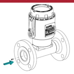
5. Clean the bearing inside surface and install the rotor in the same direction as disassembled. Slide the rotor onto the shaft and journal. Simultaneously slide the journal and rotor along the shaft to the upstream cone.
