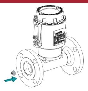
7. For NPS 1.5 meter place the thrust washer in the counterbore of the downstream cone face, polished side out. Place the downstream spring clip, cone end first, into the downstream end of housing, push the spring clip assembly into the bore contacting the journal. For NPS 2 and 2.5 meters place the downstream spring clip, small washer end first, into the downstream end of housing, push the spring clip assembly into the bore contacting the downstream cone.
