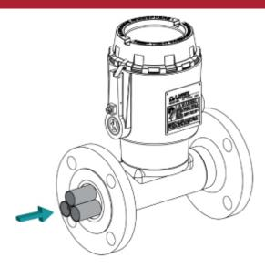
2. Insert the end of the shaft into the center hole of the upstream end of the upstream spring clip assembly. For NPS 1.5 meter, be careful not to knock the thrust washer out of the cone counterbore.
