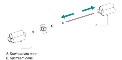
The downstream and upstream cones are welded to their respective spring clips only on NPS 1 and 1.5.
