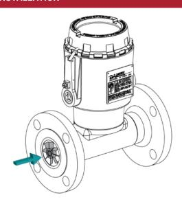
6. For NPS 1.5 meter the downstream cone is welded to the downstream spring clip assembly. For NPS 2 and 2.5 meters place the thrust washer in the counterbore on the downstream cone face, polished side out. Install the downstream cone, large diameter end first, onto the shaft and slide along the shaft to the rotor.
