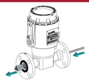
3. Pull the upstream spring clip assembly away from the downstream spring clip assembly. The shaft with the rotor and journal will stay with either the upstream or downstream spring clip assembly. Remove the downstream spring clip assembly from the upstream end of the housing.
