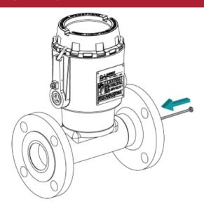
3. For NPS 1.5 meter the upstream cone is welded to the upstream clip assembly. For NPS 2 and 2.5 meters place the thrust washer in the counterbore of the upstream cone face, polished side out. Place the upstream cone, small diameter end first, on the downstream end of the shaft. Slide the shaft into the meter, contacting the downstream end of the upstream spring clip assembly.
