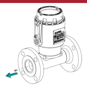
6. For NPS 1.5 meter the upstream cone is welded to the spring clip assembly.
