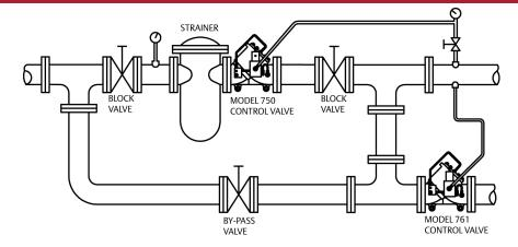
**Figure 1-5:** In this application the Model 750 pressure reducing valve lowers main pipeline pressure to a level that is within the acceptable rating of the metering equipment. The Daniel® pressure reducing valve will control a maximum reduced pressure drop of 6895 kPa (1000 psi).
