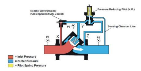
The Model 750 valves are controlled by a pressure reducing pilot that senses line pressure downstream of the valve and throttles the valve to sustain a desired maximum pressure at that point. If line pressure at the sense point begins to exceed the setting of the pilot, the pilot throttles the valve closed to maintain the required maximum pressure.
