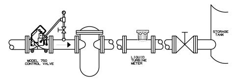
**Figure 1-6:** Pipeline "A" normally provides all product for distribution unless the pressure drops below a required minimum. At this time the Model 750 installed in an auxiliary line "B" and sensed to the main line "A", opens to maintain pressure and flow until normal main line pressure is restored.
