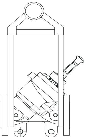
• Only use slings with ratings that exceed the weight to be lifted. Reference all safety standards for safety factors that must be included when calculating the load rating.
