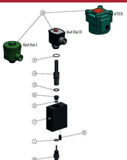
FIGURE 1-5: PARTS DESCRIPTION OF 1710 (456910) CONTROL VALVE PILOT
