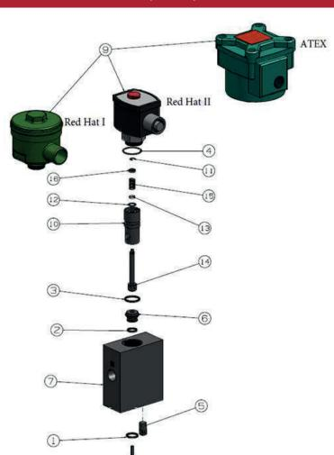
FIGURE 1-6: PARTS DESCRIPTION OF 1711 (456960) CONTROL VALVE PILOT
