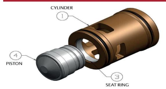
9. Turn the cylinder over with the ports on top when removing the high pressure seat ring. Remove Remove the set screw from the seat ring. Turn the seat ring counterclockwise to remove the seat ring and then remove the O-ring from the cylinder
