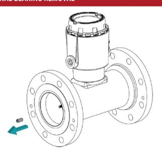
6. Remove the upstream cone from the shaft. The thrust washer should remain in the cone.
