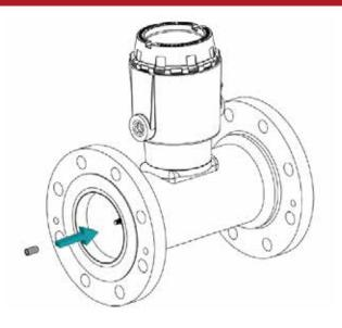
5. Install the rotor to the shaft.
