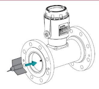
2. Thread the nut into the shaft end and insert the shaft through the upstream hanger assembly on the inlet side.
