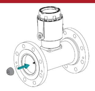
6. Install the downstream hanger assembly to the shaft.
