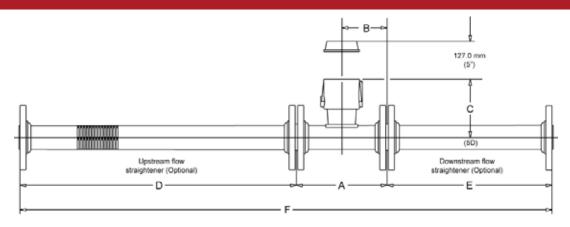
TABLE 2-11: FLOW METER AND FLOW STRAIGHTENING SECTION DIMENSIONS FOR THE SERIES 1500 LTM NPS 3-24
