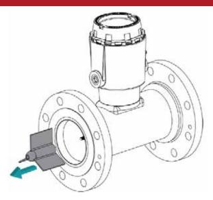
3. Remove the downstream cone from the shaft. The thrust washer should remain in the cone.
