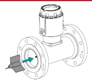
8. Install the downstream shaft nut, simultaneously holding the upstream shaft nut to prevent the shaft from turning.
