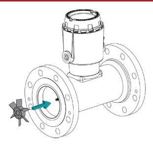
6. Install the downstream cone to the shaft. The thrust washer should remain in the cone.
