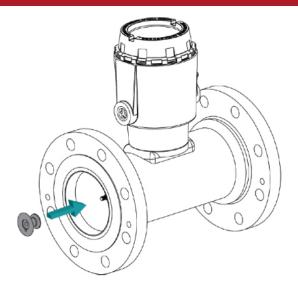
4. Insert the journal bearing in to the rotor assembly.
