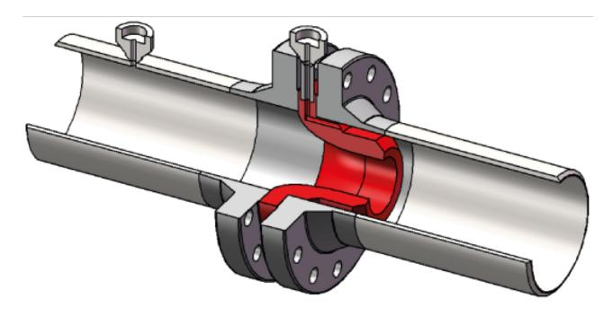
The tapped style flow nozzle is similar to the flanged design, but the downstream pressure tap is located in the nozzle. This design is recommended for smaller line sizes where the downstream tap location interferes with the holding flange or pipe weld.
