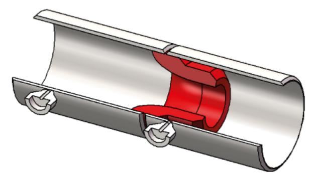
The weld-in style flow nozzle is permanently installed inside the pipe section. This is a common configuration where high temperature and high pressures prohibit the use of flanges such as in power plant feed water installations.
