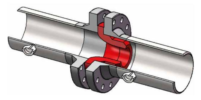
The flanged style flow nozzle is the most common design, with the nozzle inserted between pipe flanges. The pressure taps are located upstream and downstream of the flow nozzle and are located in the pipe wall. The specific location is determined by the beta ratio.
