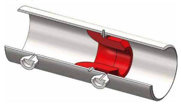
The holding ring style flow nozzle eliminates the welding of dissimilar materials. A special holding ring, of the same metallurgy of the pipe, is installed around the flow nozzle. This allows the nozzle to be made of a different material than the pipe.
