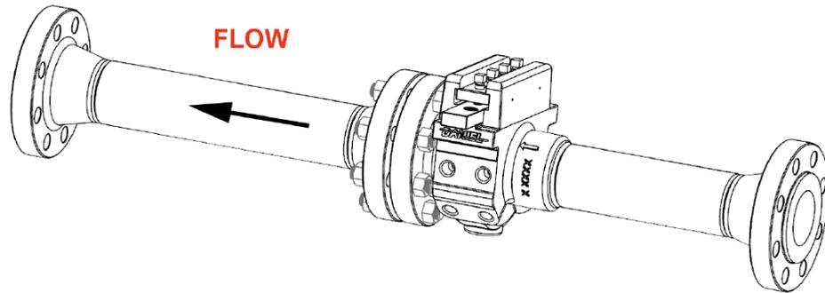
Figure 2-5: Horizontal flow - "left side" position (parallel to the ground)
