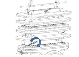
9. Using the Operating Wrench (2) rotate the Slide Valve Shaft (5) until it stops and the CLOSED position specified on the Indicator Plate (5A) is in line with the Indicator Pointer (5B).
