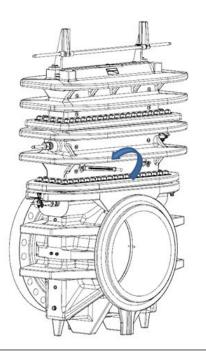
2. Wait several seconds while the pressure in the Top (14) equalizes to that of the Body (4).
