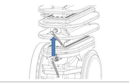
7. Rotate the Upper Plate Carrier Shaft (7) until the Plate Carrier (8DM) stops against the Sealing Bar (9 or 9HP).
