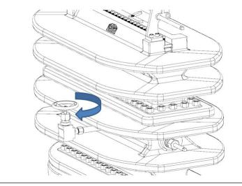
39. Open the Equalizer Valve (1) one-half to two turns with the Operating Wrench (2).
