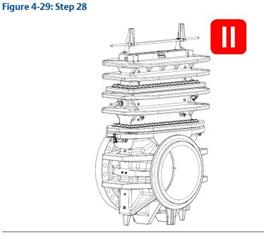
29. Using the Operating Wrench (2), rotate the Slide Valve Shaft (5) to the OPEN position.
