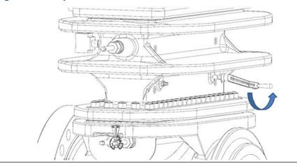
26. Return the stem to the Grease Gun (23) and begin turning it clockwise by hand into the Grease Gun (23) until resistance is felt. Once this is done, use the supplied Operating Wrench (2) to continue to turn the stem at a rate of 4 to 6 turns per minute.
