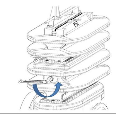
8. Close the Equalizer Valve (1) with the Operating Wrench (2).
