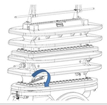
9. Using the Operating Wrench (2) rotate the Slide Valve Shaft (5) until it stops and the CLOSED position specified on the Indicator Plate (5A) is in line with the Indicator Pointer (5B).
