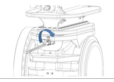
4. Rotate the Lower Plate Carrier Shaft (6) located on the Body (4) using the Operating Wrench (2) in a direction that will move the Plate Carrier (8DM) out of the Body (4) into the Top (14).
