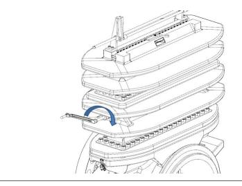
43. Rotate the Lower Plate Carrier Shaft (6) with the Operating Wrench (2) until the Orifice Plate Carrier (8DM) cannot be lowered further.
