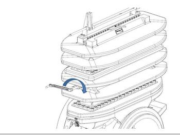
31. Rotate the Lower Plate Carrier Shaft (6) with the Operating Wrench (2) until the Orifice Plate Carrier (8DM) cannot be lowered further.
