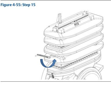
16. Once the Clamping Bar Screws (11) are loose, rotate the Upper Plate Carrier Shaft (7) located in the Top (14) with the Operating Wrench (2), until the Plate Carrier (8DM) taps against the Sealing Bar (9 or 9HP) freeing it from the Top (14).
