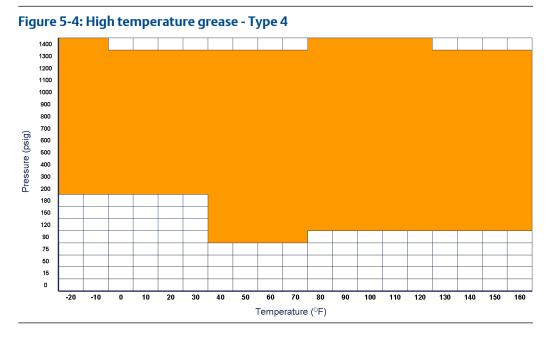
Pressure (psig) v. Temperature (°F) HIGH TEMPERATURE GREASE - TYPE 4 - Part Number:1-213- 04-103 OPTIMUM SEALING RANGE WITH NITROGEN FOR A 3" ANSI 600 SENIOR FITTING UNDER LABORATORY CONDITIONS. Colored coordinate boxes indicate no detectable leakage at that Temperature and Pressure for 30 minutes.
