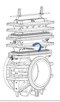
28. Wait several seconds for the Top (14) to reach pressure equilibrium with the line pressure contained in the Body (4).
