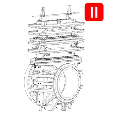
3. Using the Operating Wrench (2) rotate the Slide Valve Shaft (5) until it stops and the OPEN position specified on the Indicator Plate (5A) is in line with the Indicator Pointer (5B).
