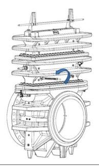
40. Wait several seconds for the Top (14) to reach pressure equilibrium with the line pressure contained in the Body (4).
