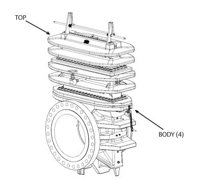
Therefore, using a Senior may eliminate the need for bypass piping, valves, and other fittings necessary with conventional orifice fitting installations. Maintenance technicians can replace and repair all parts of the Senior, including the slide valve assembly, without removing the Body (4) from the line (refer to Maintain).
