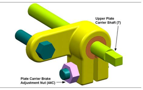
10. Rotate the Lower Plate Carrier Shaft (6), lifting the Plate Carrier (8DM) out of the Body (4). Continue to rotate the Lower Plate Carrier Shaft (6) until you visually confirm that the Upper Plate Carrier Gear Shaft (7) is rotating. Once you have visual confirmation that it is rotating, stop rotating the Lower Plate Carrier Shaft (6) and
