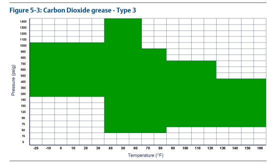
Pressure (psig) v. Temperature (°F) CARBON DIOXIDE GREASE - TYPE 3 - Part Number:1-213-04- 101 OPTIMUM SEALING RANGE WITH NITROGEN FOR A 3" ANSI 600 SENIOR FITTING UNDER LABORATORY CONDITIONS. Colored coordinate boxes indicate no detectable leakage at that Temperature and Pressure for 30 minutes.
