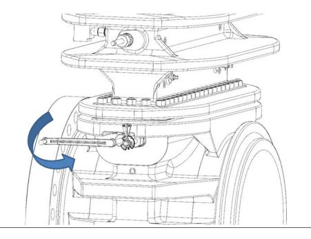
5. Continue to rotate the Lower Plate Carrier Shaft (6) located on the Body (4) until the Upper Plate Carrier Shaft (7) located in the Top (14) begins to rotate.
