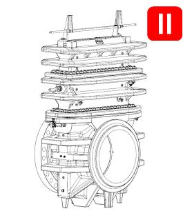
3. Using the Operating Wrench (2) rotate the Slide Valve Shaft (5) until it stops and the OPEN position is specified on the Indicator Plate (5A) with the Indicator Pointer (5B).
