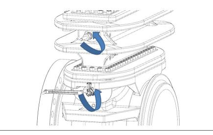
6. Move the Operating Wrench (2) from the Lower Plate Carrier Shaft (6) to the Upper Plate Carrier Shaft (7).
