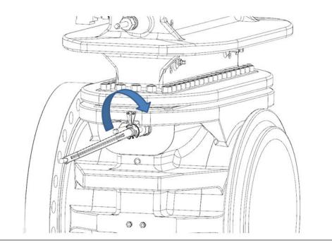
4. Rotate the Lower Plate Carrier Shaft (6), located on the Body (4), using the Operating Wrench (2) in a direction that will move the Plate Carrier (8DM) out of the Body (4) into the Top (14).
