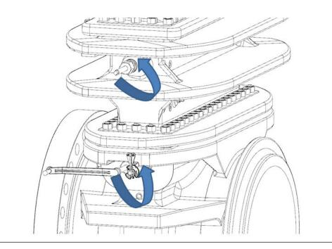
6. Move the Operating Wrench (2) from the Lower Plate Carrier Shaft (6) the Upper Plate Carrier Shaft (7).
