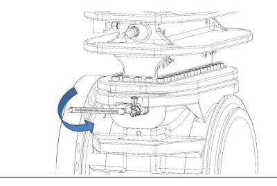
5. Continue to rotate the Lower Plate Carrier Shaft (6) located on the Body (4) until the Upper Plate Carrier Shaft (7) located in the Top (14) begins to rotate.
