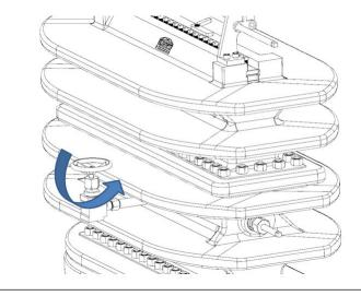
Steps 25 and 26 are ONLY required for the Seniors equipped with grease assisted, metal-tometal slide valves. Personnel operating Seniors equipped with O-Ring seal "soft seat" design slide valves skip to step 26.
