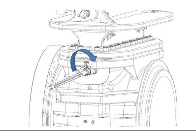
30. Rotate the Upper Plate Carrier Shaft (7) with the Operating Wrench (2) in the direction to lower the Orifice Plate Carrier (8DM) into the Body (4).
