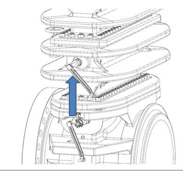
7. Rotate the Upper Plate Carrier Shaft (7) located in the Top (14) until the Plate Carrier (8DM) stops against the Sealing Bar (9, 9HP).
