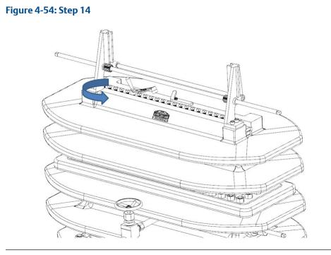
Once the Clamping Bar Screws (11) are loose, rotate the Upper Plate Carrier Shaft
