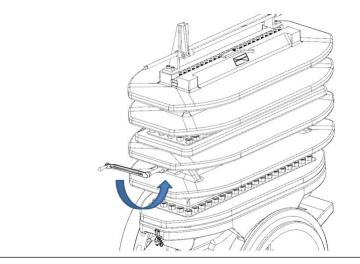
30. Slide the Clamping Bar (12 or 12HP) containing the Clamping Bar Screws (11), the Sealing Bar (9) from the Top (14).
