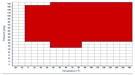
Pressure (psig) v. Temperature (°F) STANDARD GREASE - TYPE 1 - Part Number: 1-213-04-001 OPTIMUM SEALING RANGE WITH NITROGEN FOR A 3" ANSI 600 SENIOR FITTING UNDER LABORATORY CONDITIONS. Colored coordinate boxes indicate no detectable leakage at that Temperature and Pressure for 30 minutes.
