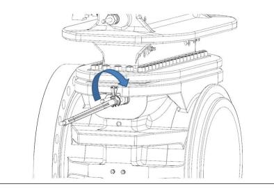
42. Rotate the Upper Plate Carrier Shaft (7) located in the Top (14) with the Operating Wrench (2) in the direction to lower the Orifice Plate Carrier (8DM) into the Body (4).
